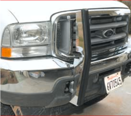
The cross bars are then bolted into position on the upright brackets. The cross bars come pre-assembled and simply bolt in at the rear.
