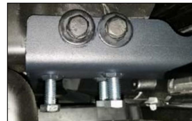
Passenger side of either frame view of mounting hardware for mounting brackets installed on frame
