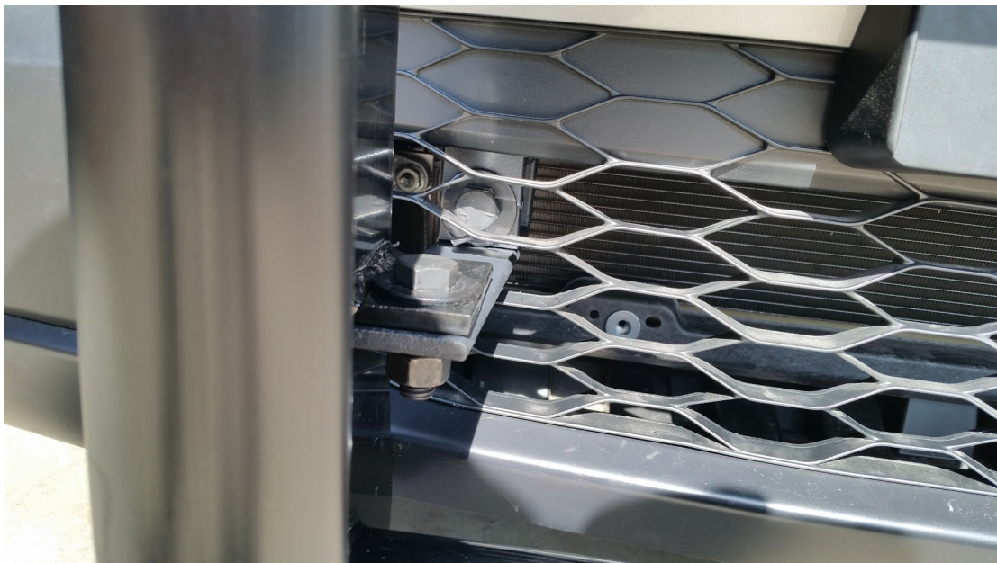
Example of Cutout in Lower Grille for Bracket
